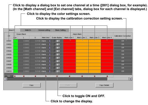
Enter external input channel settings in the same manner as those of the measurement channel items. Also note that this measurement channel setting screen is only one example; your actual screen may vary.
