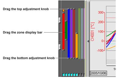
You can change the waveform display zone on the trend display screen by clicking the edit zone icon on the tool bar or by selecting [Y-Axis] - [Edit Zone] in the menu bar. The size of the zone can be changed by dragging the top and bottom adjustment knobs. The entire zone can be moved by dragging the zone display bar.
