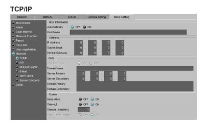
Set the IP address to a fixed IP address or obtain it automatically (DHCP). Consult with your network administrator for the network parameters such as the IP address, subnet mask, default gateway, and DNS.
