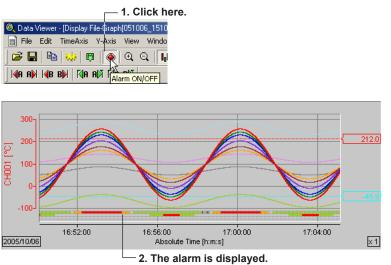
The alarm conditions of alarm 1 to 4 are displayed in the alarm display area.
