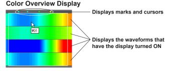
The measured values of the entire data are displayed using various colors. By assigning 50 different colors from the minimum to the maximum values of the scale, the measured values are assigned to those colors.
