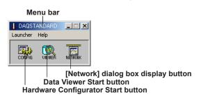
After installing the software, when you first start it, the [Network] dialog box appears. For details about the setting method, see section 2.3, "Setting the Communication Method". If the DX1000/DX2000 is not turned ON or connected when the communications settings are completed, the [Network] dialog box opens.
